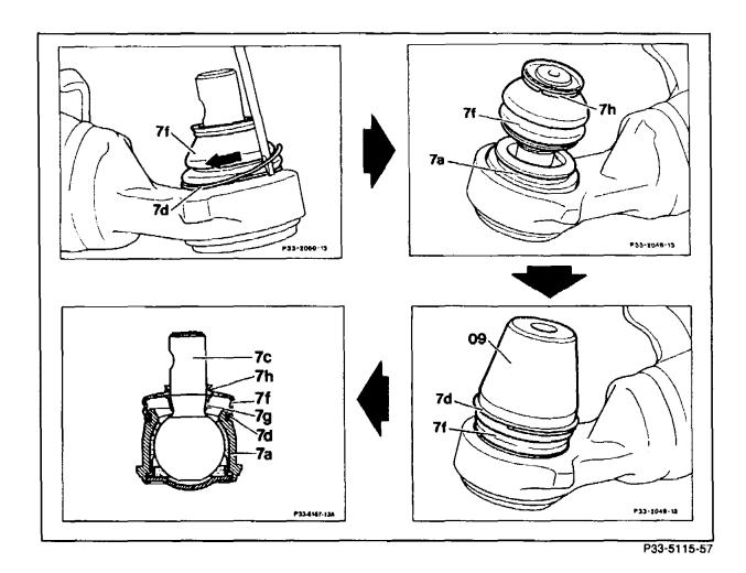
Wire clamping ring (7d) . . . . . . . . . . Remove, install.
