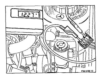
9 Level adjustment switch (S77) in "lowered level" position.
