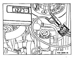
5 Level adjustment switch (S77) in "raised level" position.
