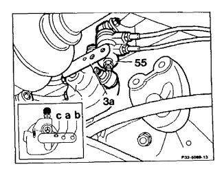
11 Check oil level in oil reservoir and top up if necessary.
