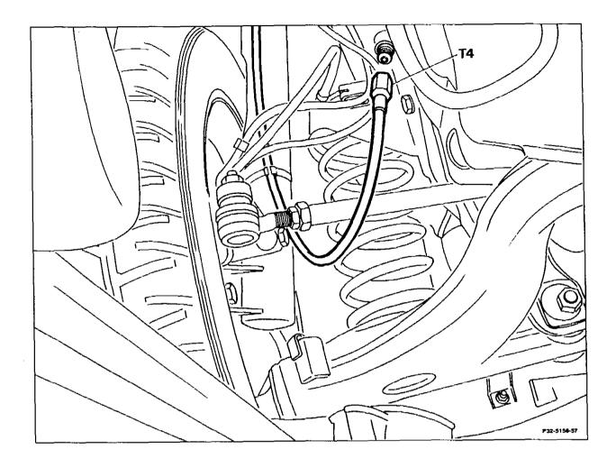
Return line (T4) . . . . . . . . . . . . . . . Detach, attach at connection of steel line to leak oil hose.
