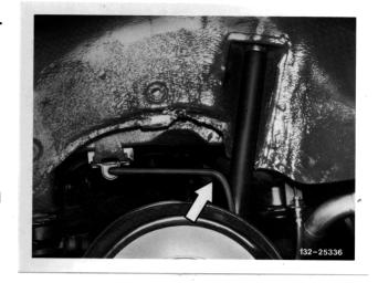
12 Fasten torsion bar to frame floor with mounting bracket on left and right. Tightening torque for new self-locking hex. head bolts 20 Nm.
