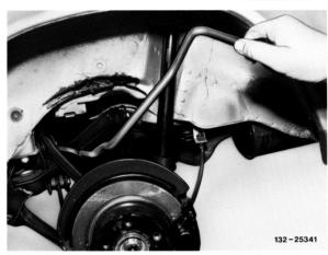
9 If it is also necessary to remove the connecting rod, remove it after screwing off the hex. head bolt with nut (arrow) (spring link cover removed).
