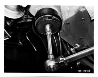
8 Lower rear axle slightly and remove torsion bar to left after turning as required.
