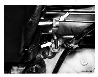
7 Unscrew both hex. head bolts for rear axle front mount on frame floor while supporting rear axle center assembly with car jack.
