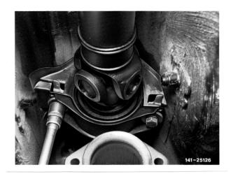
5 Separate propeller shaft from rear axle center assembly.
