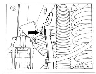
3 Unscrew hex. head bolts for torsion bar mount on frame floor, remove rubber mount.
