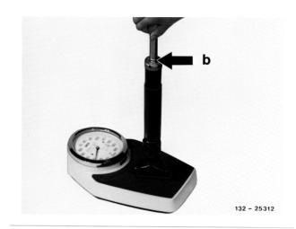
In the event of a gas or oil leak the extension force of the piston rod is reduced. If the value is less than the minimum value, the shock absorber can no longer function properly and should be replaced.
