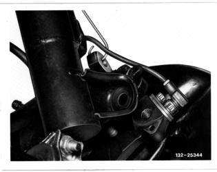
8 Remove suspension parts: stop buffer (11h).
