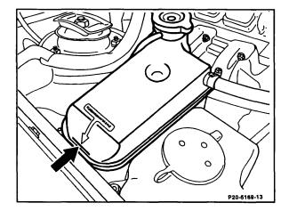
On vehicles without separate expansion tank, up to marks as illustrated.
