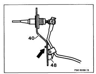
Accelerator pedal remove, install (30-1321). Footwell trim ...... remove, install. Return spring (35) ..... detach, attach. remove from accelerator pedal lever (33), fit on. Bowden cable (30) .....
