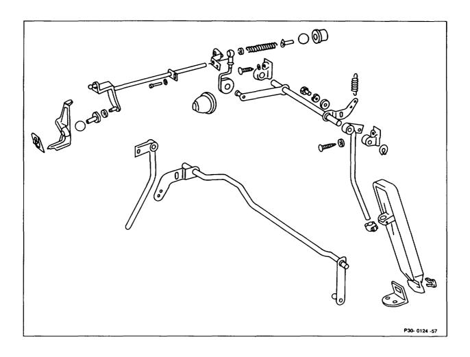
Chassis accelerator control shaft ..... remove, install (30-0320).
