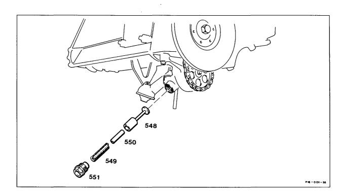
Screw plug (551) ..... remove, screw on (50 Nm)
