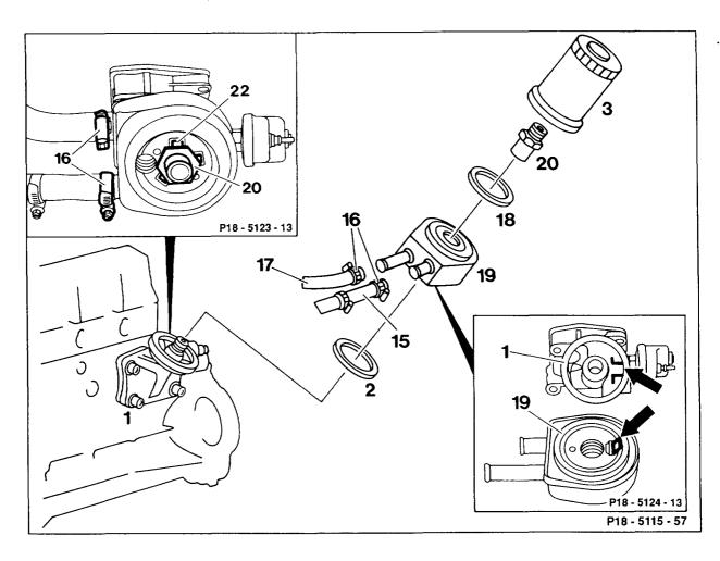
Coolant at crankcase drain, pour in (20-0100). Replaceable cartridge (3) remove, install (18-0020) with wrench socket 103 589 02 09 00. Hose strap (16) ..... slacken, tighten. Securing tab (22) ..... bend up. Sleeve nut (20) unscrew. Oil heat exchanger ...... detach from cooling hoses (15) and (17), remove, install. Installation notes Gasket (2) of heat exchanger (19) ..... replace.
