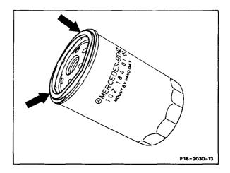
7 Screw on replaceable cartridge (579) and tighten by hand.
