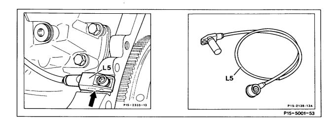
Screw (arrow) Crankshaft position sensor (L5) ......
