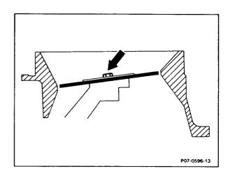
2 Center air flow sensor plate. To do this, remove fuel pump relay and briefly bridge the two contacts 7 and 8, on model 129 engine systems control unit MAS between contacts 1 and 2, for (USA) (J) as of model year 1990 at KE control unit (N3) between sockets 11 and 20 to build up pressure.
