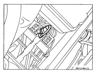
Check with a feeler gauge (approx 0.5 mm) that the air flow sensor plate is accurately centered. The air flow sensor plate must also not stick even if slight pressure is applied to the side (bearing play eliminated). Tighten securing bolt to 5-5.5 Nm and install
