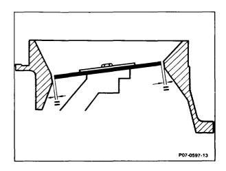
Check zero position (rest position) of sensor plate. The top edge of the sensor plate must be flush with the top edge of the cylindrical part (arrow) on the air funnel. It is permissible for the plate to be higher by not more than 0.2 mm.
