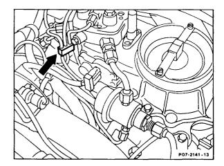
3 Connect fuel pressure hose to fuel distributor and hold in measuring glass or beaker.
