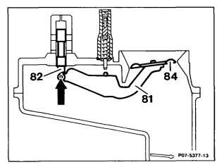
5 Check control plunger in fuel distributor for leaks.
