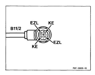
Coolant temperature sensor Coupling pin assignment:
