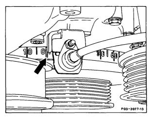
Position marking (22) or position hole of camshaft must be aligned with the marking (517) on 1st camshaft bearing.
