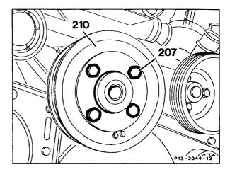
6 Install holding lock for crankshaft/ring gear (30-5000).
