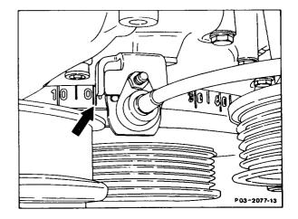
3 Slacken bolts (207) of belt pulley (210) of viscous fan clutch.
