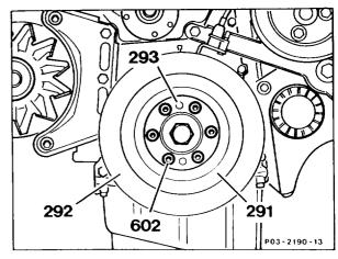
8 Unscrew bolt of hub with 3 dished springs.
