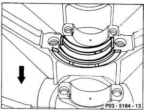
6 Install axial bearing in crankshaft bearing point 5.
