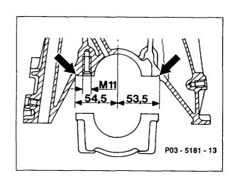
The forged conrods are guided axially in the pistons (piston-guided conrod) (arrows).
