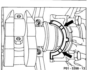
9 Coat conrod bearing shells with engine oil and install bearing caps.
