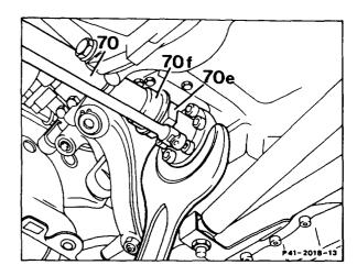
10 Unbolt front axle shafts (59). Operate footbrake in order to slacken the six bolts.
