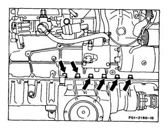
21 Lower front axle housing as far as possible. Unscrew bolt for sprocket (1) and take off sprocket (1). Unscrew bolts (arrows) and take out oil pump downward. Take off front axle housing to the rear. Pay attention to drive chain of oil pump.
