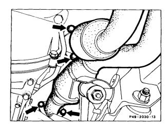
9 Unbolt propeller shaft (70) to front axle at front axle housing. To do this, counter-hold the connecting flange with 65 mm open-end wrench and unscrew six bolts.
