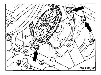
22 Clean contact surfaces on front axle housing. Apply sealant 001 989 45 20 10 to the contact surface on front axle housing (a = silicon bead  $\emptyset$  1.5 mm). First mate front axle housing to the transmission, then bolt to crankcase.
