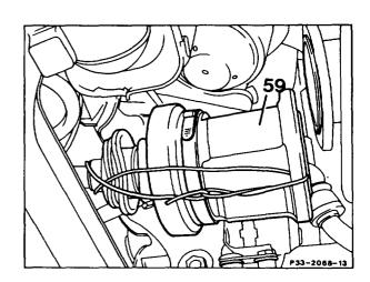
12 Unplug connector (arrow) of the oil level sensor on the left at oil sump and at front axle housing, respectively.
