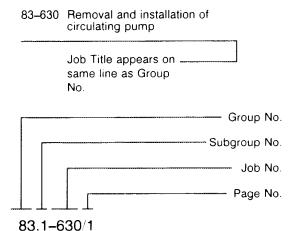
Technical data, tightening torques and tools are listed at the beginning of each job.
